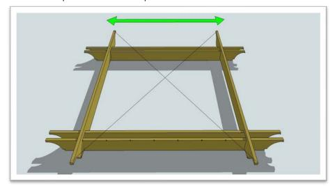
Move one set of the beams from side to side until you have the same measurement both ways. When you have the same measurement, it is perfectly square. Once square, make sure the assembly does not move.
