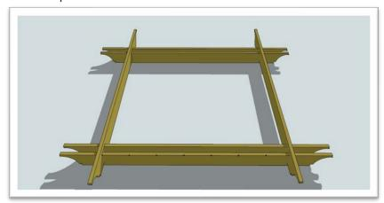
• **Step 4** - To ensure the assembly is square, hook one end of a tape measure on the outside tip of the rafters and pull the tape to the opposite corner. Write down the measurement. Then repeat for the opposite corner like this. This is easier if you and your helper both have a tape measure and pull them across at the same time.
