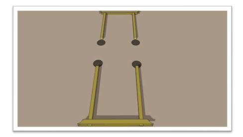
• **Step 13** - With one person at each post, tilt one assembly up, lift and drop the posts into the postholes, or into the post bases if on concrete. Have your helper(s) hold the assembly plumb.
