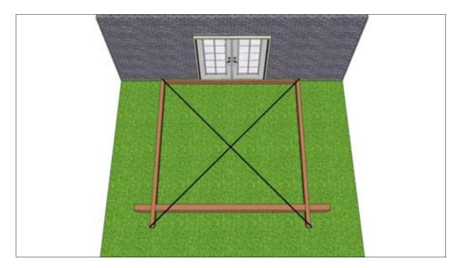
Ensuring the ledger board remains in place, move the beams from side to side until you have the same measurement both ways. When you have the same measurement, it is perfectly square. Once square, make sure the assembly does not move.
