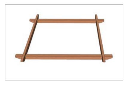
**Step 4** - To ensure the assembly is square, hook one end of a tape measure on the outside tip of the rafters and pull the tape to the opposite corner. Write down the measurement. Then repeat for the opposite corner as shown below. This is easier if you and your helper both have a tape measure and pull them across at the same time.
